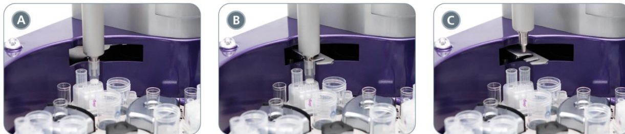
Figure 8. Tip Strip Process. (A) The robotic arm places the used 5 mL tip partly back into the tip rack. (B) The tip stripping arm swings out to engage the tip head just above the 5 mL tip. (C) The robotic arm moves up and the tip fully falls into the tip rack.
